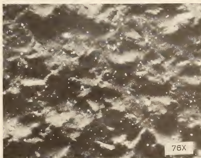
Figure 3.2.2 Corrosion of absorber material D sample from a full-size collector after 480 exposure days ( \geq 17,000 kJ/sq-m-day)
