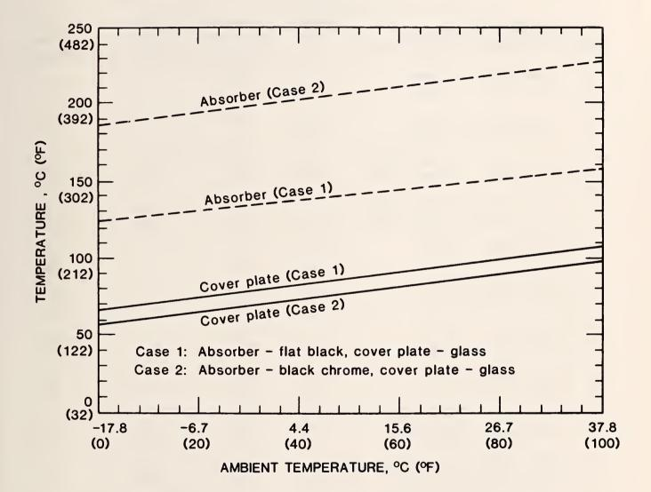
Figure A.1. Calculated surface temperatures of absorber and collector cover plate(s) under conditions of stagnation. Fixed meteorological, operational and optical parameters are given in tables A.2 through A.5. The surface temperatures for the absorber and cover plates are also presented in table A.1 at ambient temperatures of -17.8 and 37.8°C.
