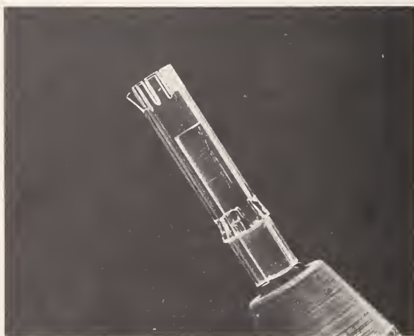
Figure 4. Silica-glass former on holding jig for flame working. Some of the "fingers" have been flame polished and flared.
