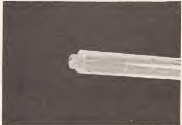
Figure 2. Silica-glass former tubing potted in close-fitting borosilicate glass holding tube with hard wax compound.
