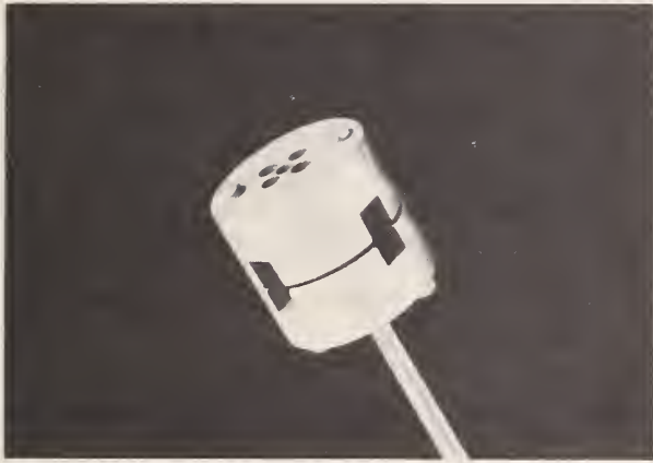
Figure 5. Stainless steel hole locating jig (supported on a rod for illustration). A silica-glass disk is clamped between the two halves of the jig, and holes are drilled with abrasive powder propelled by air from a nozzle inserted into the locating holes in the jig. The rectangular openings are exhaust ports for the spent abrasive.
