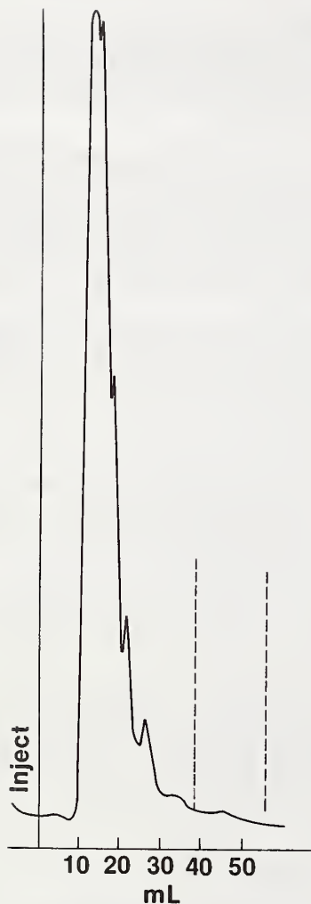
Figure 6. Prefractionation of an Oil on \mu Bondapak-NH 2 . Mobile Phase: 5 Percent Methylene Chloride in Hexane.
