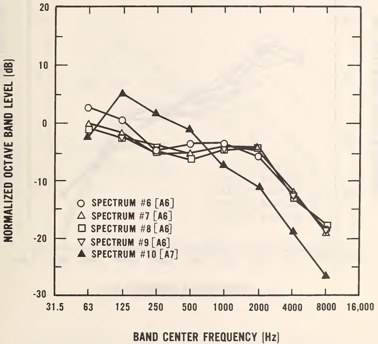
Figure A7. Normalized "average" traffic noise spectra at 15 m.
