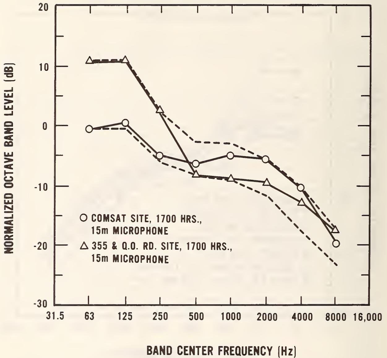
Figure A11. Range of normalized octave band levels for each of the seven actual traffic noise recording sites of Section 2.1 at the 15-m microphone position.
