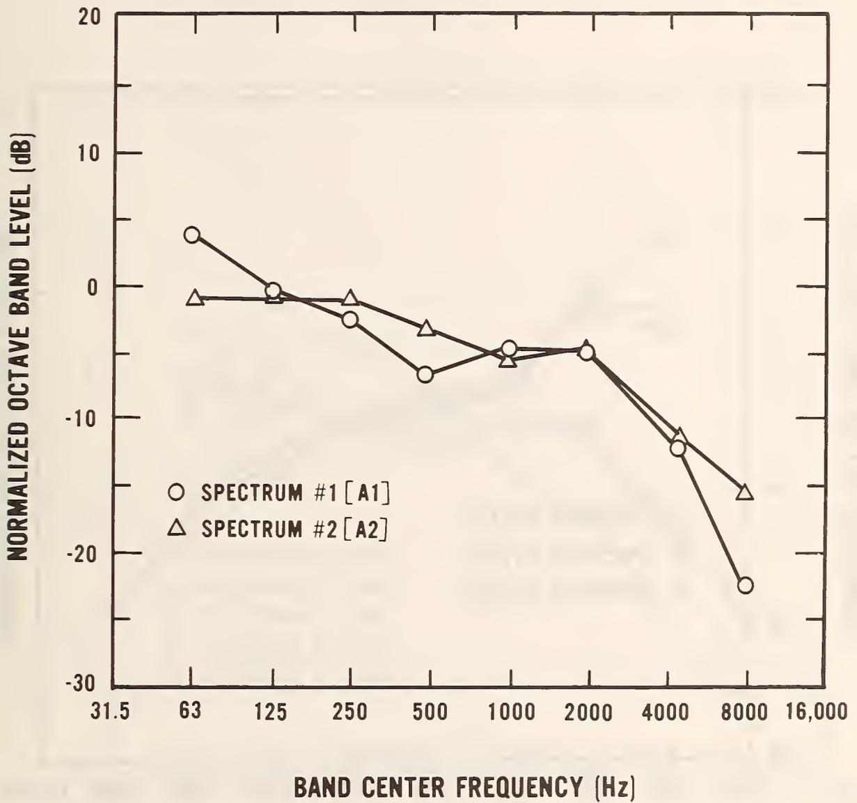
Figure A5. Normalized "average" traffic noise spectra at 7.5 m.
