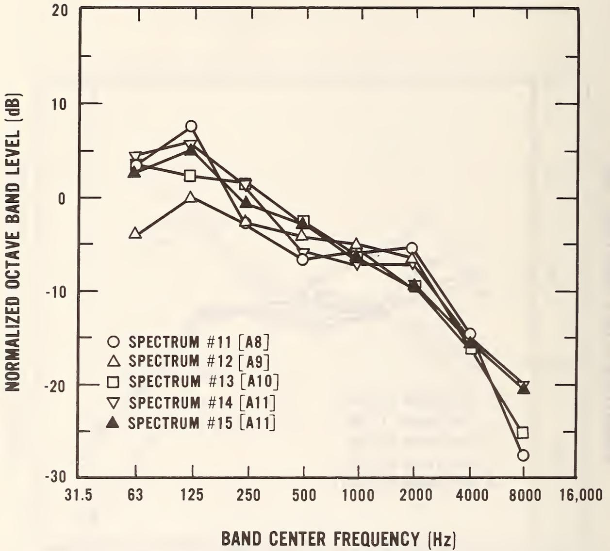
Figure A8. Normalized "average" traffic noise spectra at 30 m.
