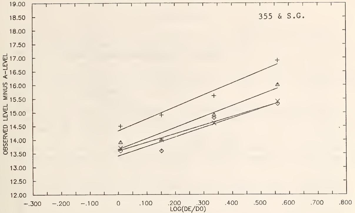
Figure 9. Difference between the Mark VI Loudness Level and the A-weighted sound level, as a function of effective distance, for the four recording times at the 355 & S.G. intersection.
