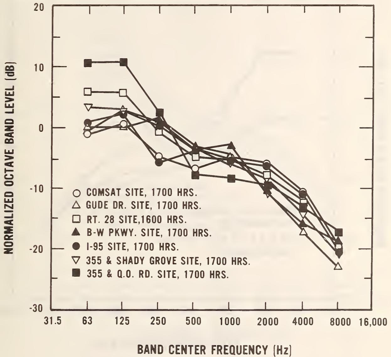
Figure A10. Normalized LEQ octave band spectra for each of the seven actual traffic noise recording sites of Section 2.1 at the 15-m microphone position.
