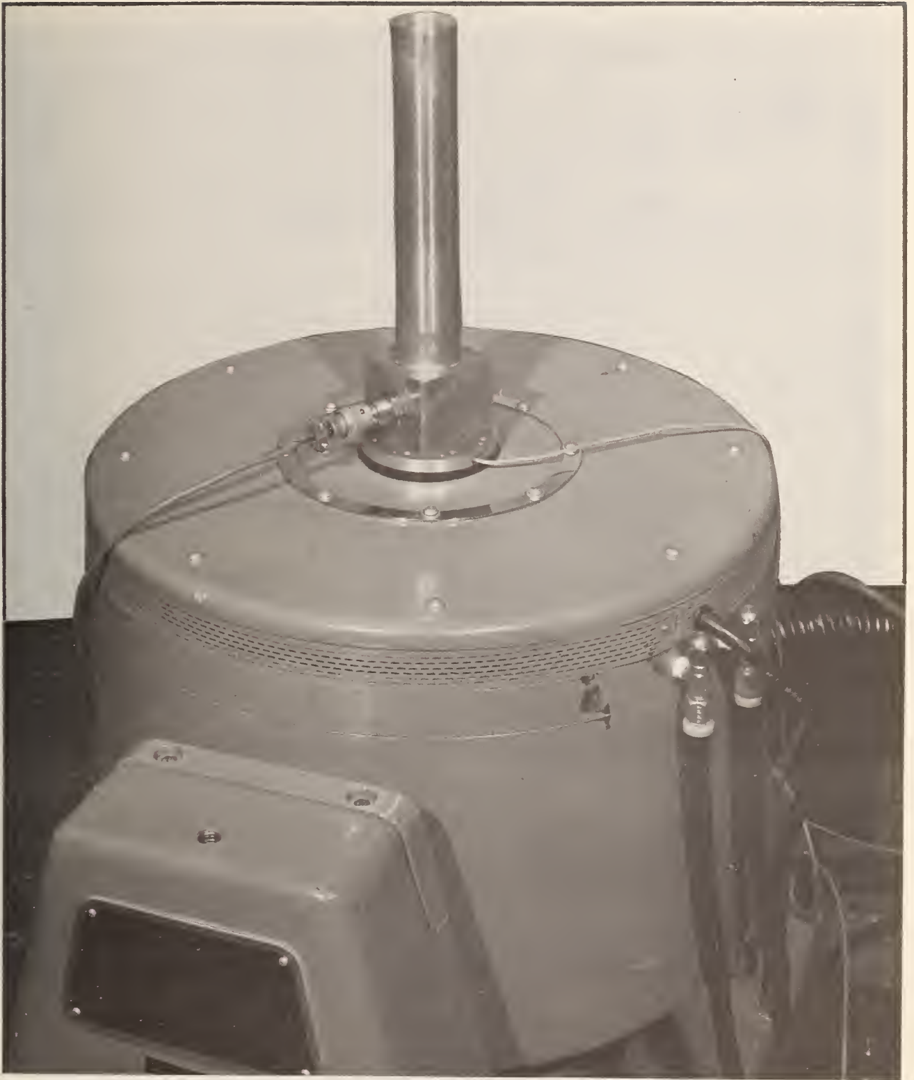
Figure 13. Liquid-medium sinusoidal pressure calibrator, with transducer to be calibrated, is shown mounted on an electrodynamic vibration exciter.
