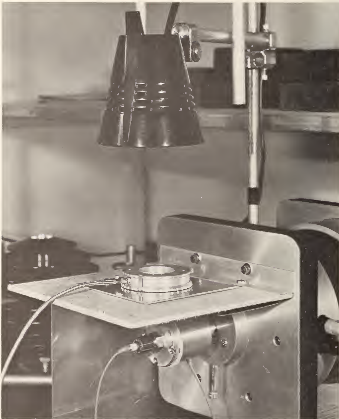
Figure 16. Experimental set-up for investigation of effects of thermal transients on performance of piezoelectric accelerometers showing radiant heat lamp and shutter with test-accelerometer side exposed to thermal transient.
