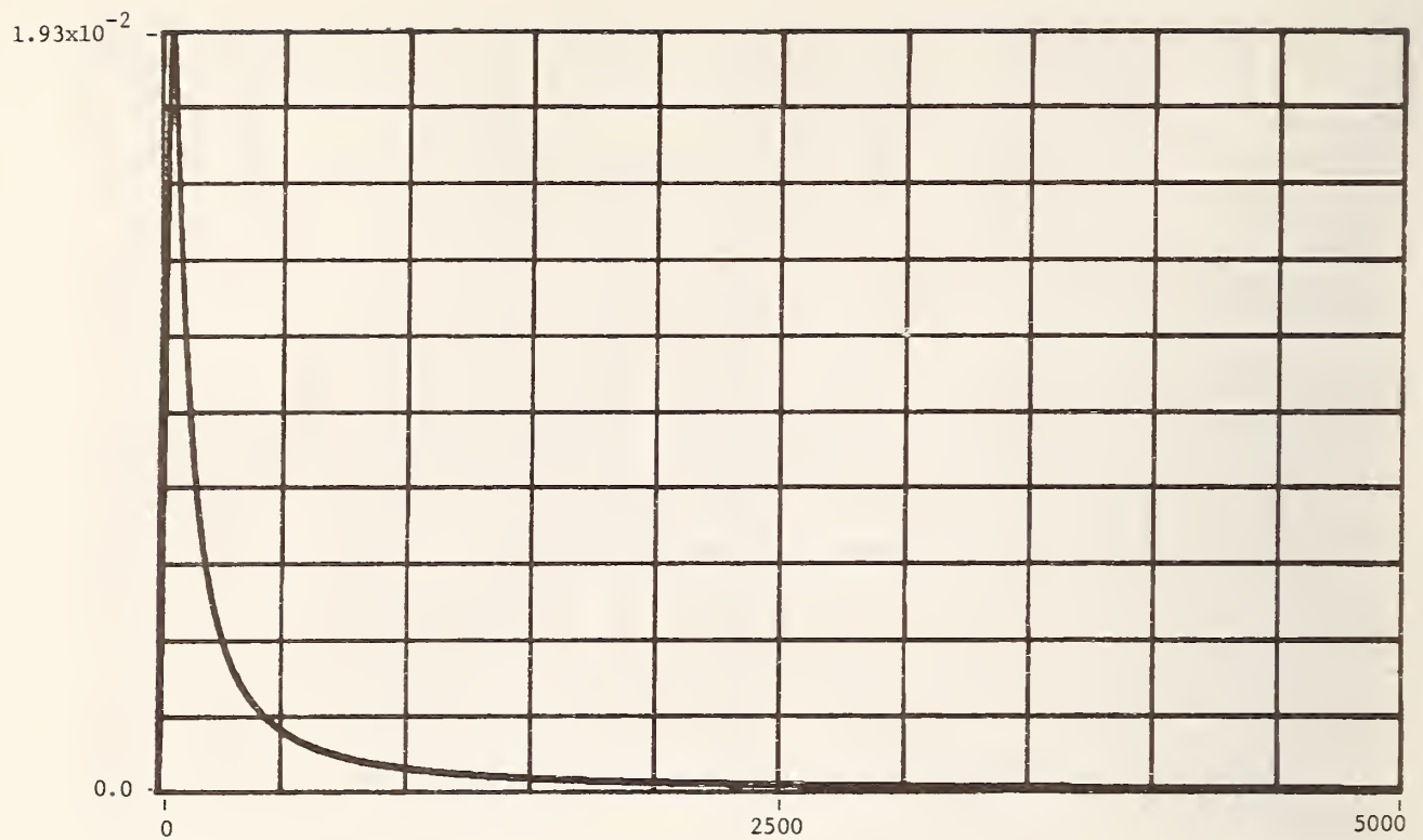
Figure A-65. Modeled and computed time domain impulse response for 304.8 meters (1000 ft) of E. Ordinate units are seconds -1 , abscissa units are nanoseconds and time spacing between points is 4.883 ns.
