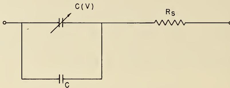
TYPICAL  $\left\{ \begin{array}{l} C = 0.4 - 2.0 \mu\mu f \\ R_s = 0.8 - 5.0 \text{ OHMS} \end{array} \right.$
