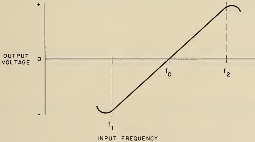
(B) THE OUTPUT VOLTAGE AS A FUNCTION OF INPUT FREQUENCY
