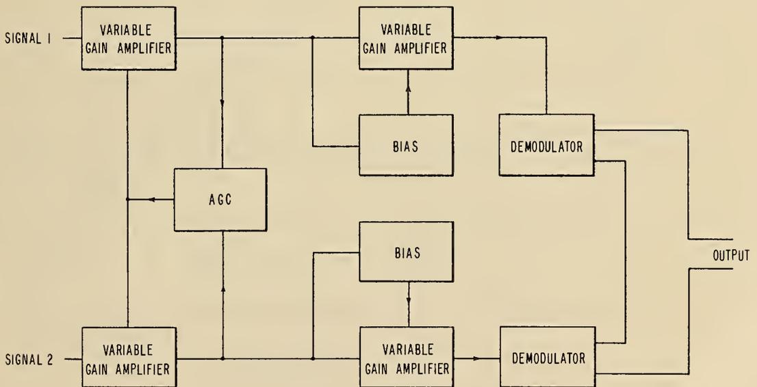
(c) MAXIMAL RATIO COMBINER (PRE-DETECTION)
