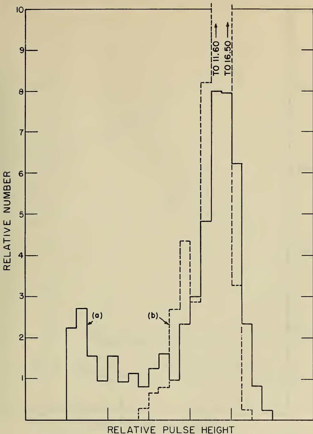
Fig. 9. Pulse height distributions, experimental and calculated. Curve (a) Pulse height distribution obtained experimentally with Pilot B-Li 6 I spectrometer and 14.1 Mev neutrons. Curve (b) Pulse height distribution calculated by Leiss for Boron-10 loaded liquid scintillator and 10 Mev neutrons.
