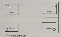
(b) A shift test load shall be conducted using a one-half nominal capacity test load centered as nearly as possible, successively at the center of each quarter of the load-receiving element as shown in the diagram below,
