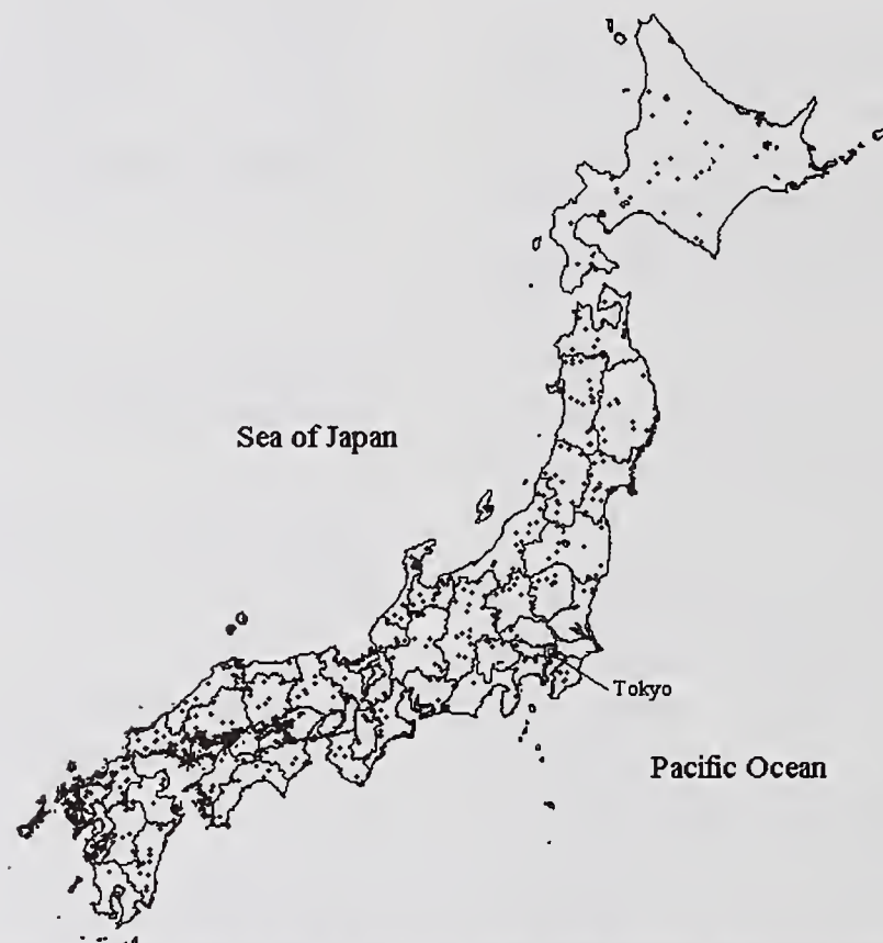
Figure 1 Distribution of dams where seismograph installation is completed
