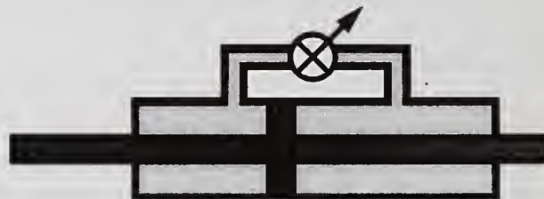
Figure 1. Schematic of Variable-Orifice Damper.
