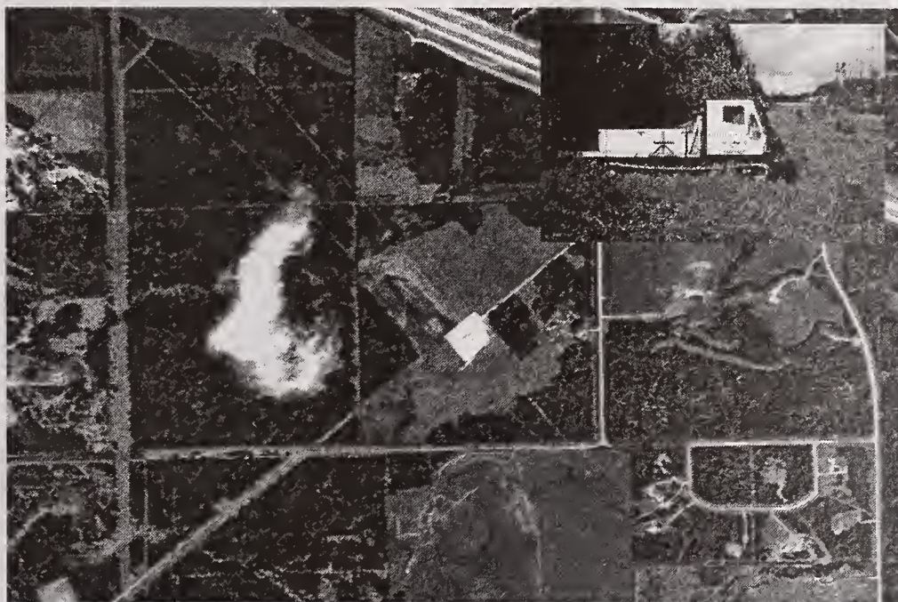
Figure 4: Unauthorized intrusion detection on Canadian pipeline using satellite imagery
