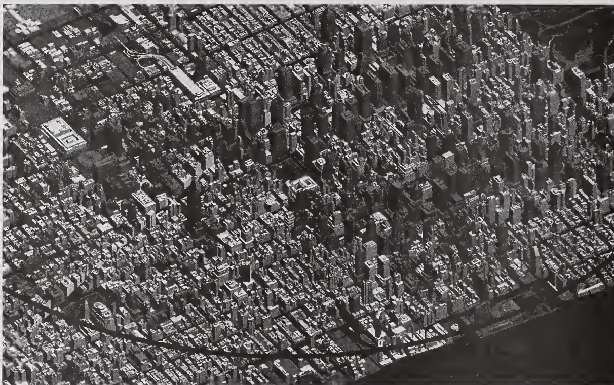
Figure 1. Sample LiDAR data set of the downtown New York area collected by EarthData. The vertical accuracy is about .8 feet on average across the data set.
