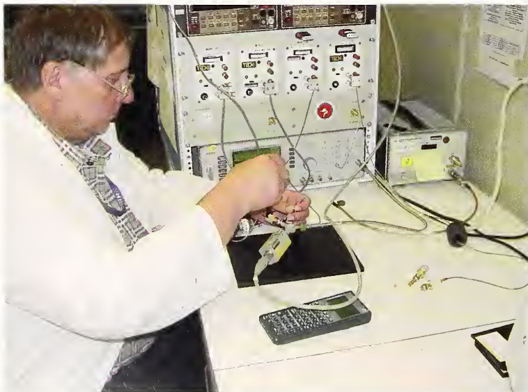
NIST direct comparison 2.4 mm power measurement system at NPSL.
