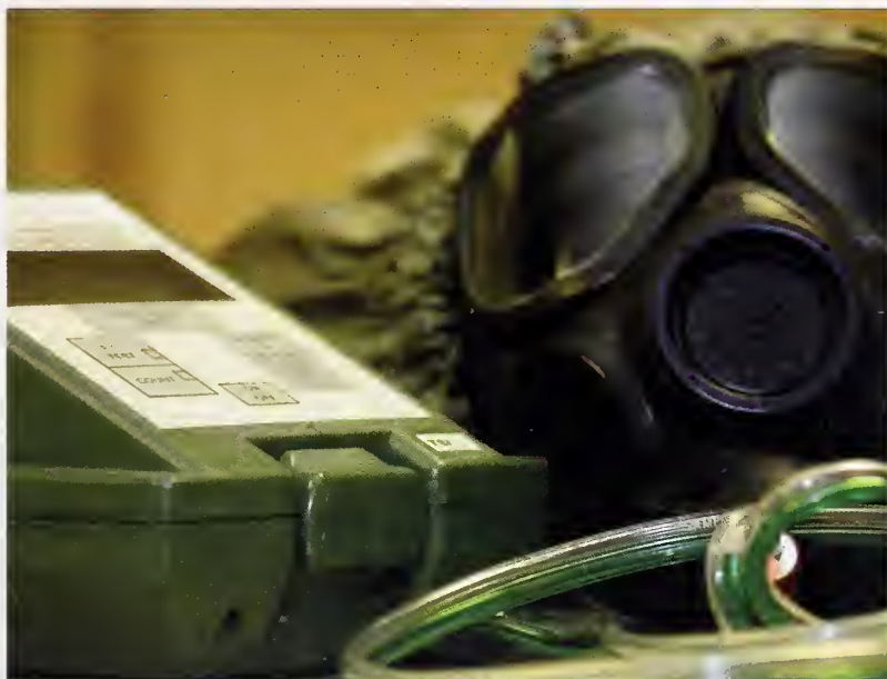
The M41 tester connected to gas mask that is mounted on a mannequin head. (Courtesy of TSI, Inc.)
