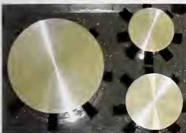
Prototype aluminum cylinder set used to calibrate static RCS measurement systems in the frequency range of 2 to 18 GHz. The cylinders are manufactured to a tolerance of \pm 0.0127 cm.
