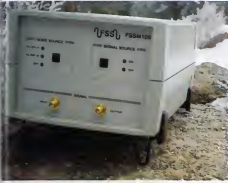
Commercial phase noise standard licensed by NIST. (Courtesy Femptosecond Systems.)
