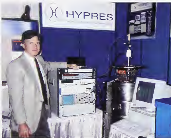
Transportable commercial Josephson junction voltage standard.
