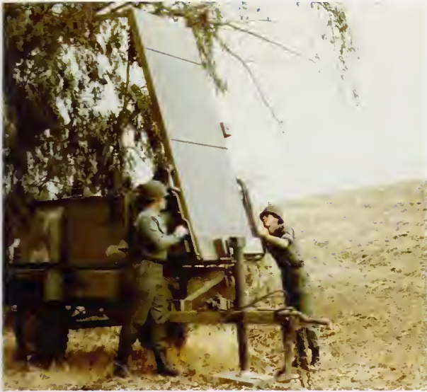
Army mortar firefinder array antenna.
