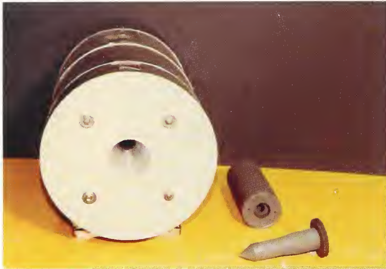
NIST constructed, high-temperature blackbody (zinc melting point).
