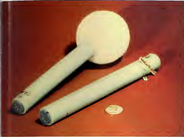
NIST three orthogonal dipole electric field intensity probe.
