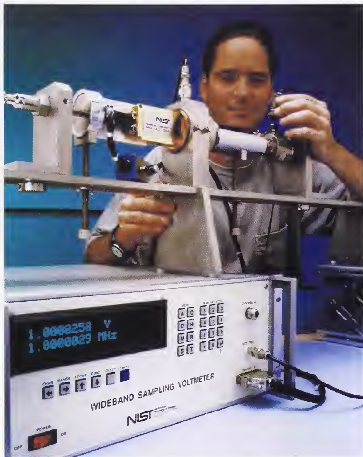
NIST wideband sampling voltmeter comparing RMS voltage readings with a thermal voltage converter standard.
