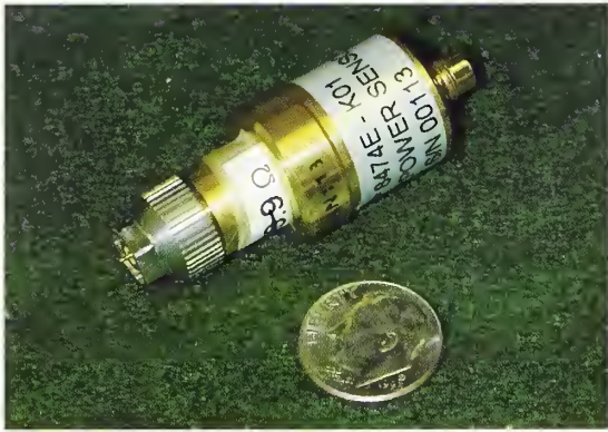
NIST 2.4 mm transfer power detector (shown next to dime).
