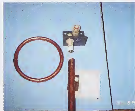
NIST fiber-optic-coupled E and H probe.
