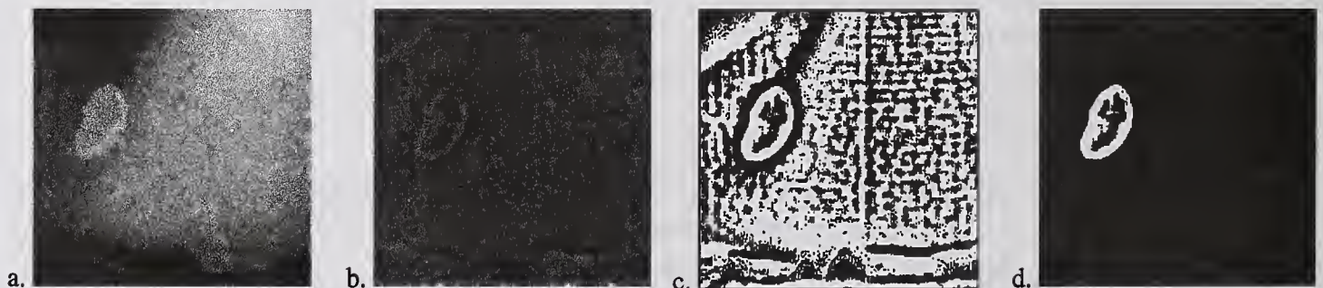
Figure 4: Image processing: a.) Original image b.) Image with contrast enhancement and shading corrections c.) Image after threshold segmentation d.) Image with detected and classified object
