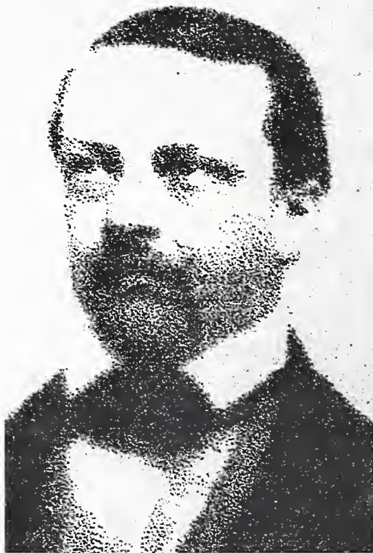
Figure 13. A pointillist portrait of William Helmholtz, painted with high-velocity krypton ions. Each dot is formed by the impact of an individual ion. The width of the head is approximately 250\ \mu\text{m} , about twice the width of a human hair. Figure courtesy of B Fischer (Fischer and Metzger 2000).
