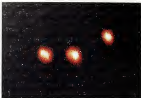
FIGURE 1. AFM image showing the topography of three \text{Xe}^{44+} impact sites on mica. The image is 50 nm x 80 nm and the features are approximately 20 nm in diameter and 1 nm high.
