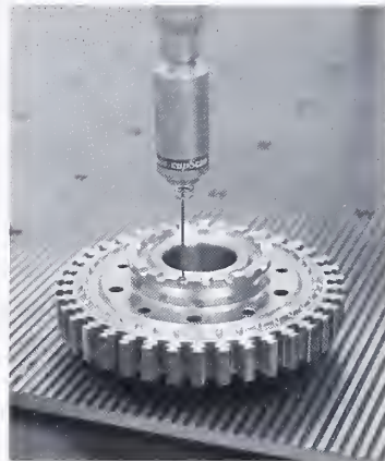
Figure 20. Inspection Workstation team members successfully used the computer-aided design (CAD) data file for a part to generate a control program for driving the Coordinate Measuring Machine's delicate probe. (Photo collection, AMRF Files, NIST)
