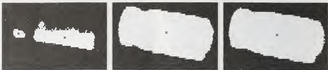
(a) 10 sec. (b) 60 sec. (c) 180 sec. Fig.3 Growth of high temperature cluster of electric radiant heater (Number of second is elapsed time from turn on the heater)
