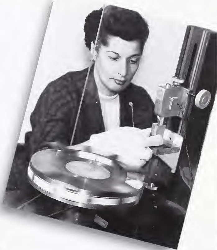
Tests performed with this mechanical comparator provided data on the stability of gage blocks developed by NIST.
