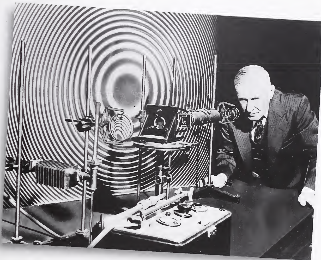
NIST made this mercury lamp available to science and industry as an ultimate standard of length in 1951. Length measurements were based on the circular "interference fringes" seen in the background.
