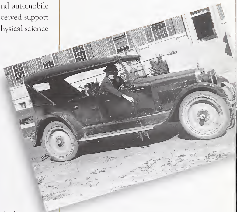
This car, rigged with two pistols, was used to measure a motorist's reaction time in applying the brakes.
