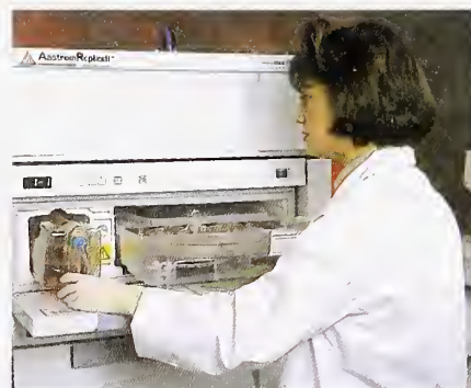
Inserting Cell Cassette into Incubator.
