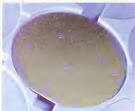
A wafer populated with arrays of vertical cavity surface emitting lasers.
