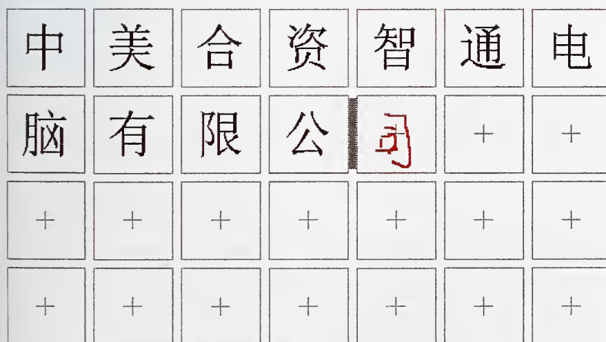
A screenful of Chinese characters, with one in the process of being composed. They were entered into the computer after being written on a pad using a stylus.
