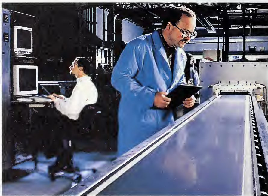
A large area solar grade silicon sheet emerging from a silicon growth reactor which incorporates new ATP-funded technology.
