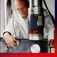
An ultrasonic strain gauge (above) was developed by MSEL researchers for in-service inspection of bridges. A small company recently commercialized the technology as a portable instrument, which is being sold to state highway departments.
