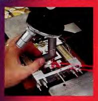
NIST researchers are refining a technique called electronic speckle-pattern interferometry to measure deformation during the mechanical testing of thin films for electronics applications. A bright laser is directed at a material, and the reflected pattern, captured by a digital camera, changes during the deformation process.
