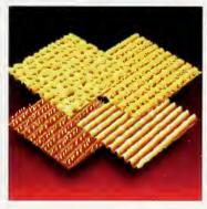
Atomic force microscopy is an emerging method for evaluating thin film surfaces. MSEL researchers use it to produce images of polymer blends separating to follow chemical or physical patterns on surfaces. Scientists can produce patterns using different materials to assess surface properties and interactions between materials.
