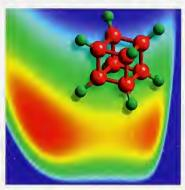
Neutron studies of molecular structure and vibrational states help scientists model and understand materials such as cubane, a synthetic, cubeshaped carbon array that may have biomedical applications. Cubane contains unstable, high-energy bonds between atoms (the green areas in the computer model above).
