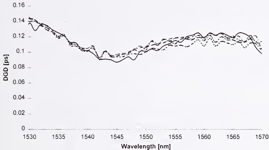
Fig. 3 PMD of a commercial EDFFA; DGD curves measured at different power levels and different measurement settings
