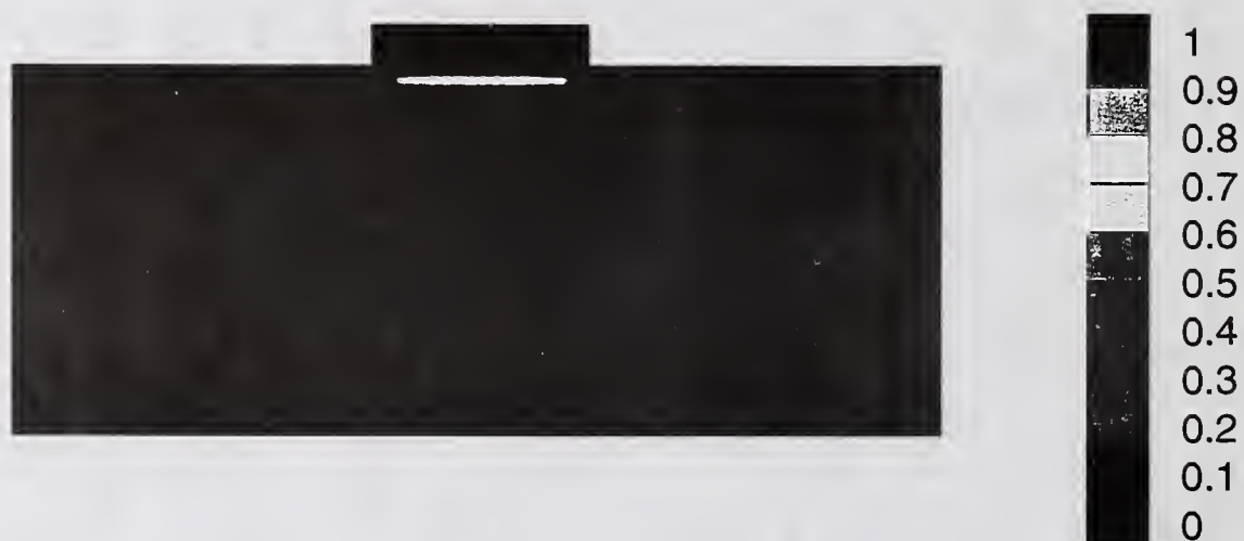
Figure 6 Predicted martensite distribution (volume fraction)
