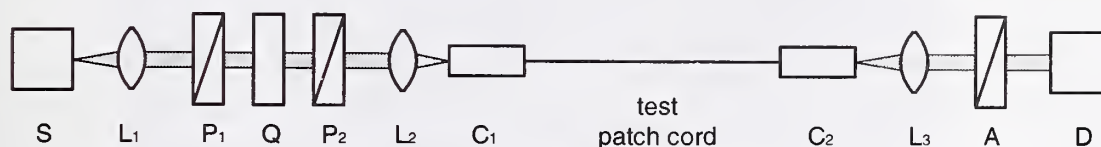
Fig. 1. The experimental configuration for the direction of PA and the ER measurement
