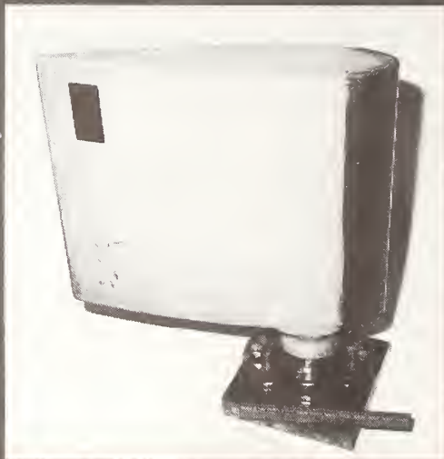
Figure 2. Composite Control Surface (1/4 - Scale Prototype)
