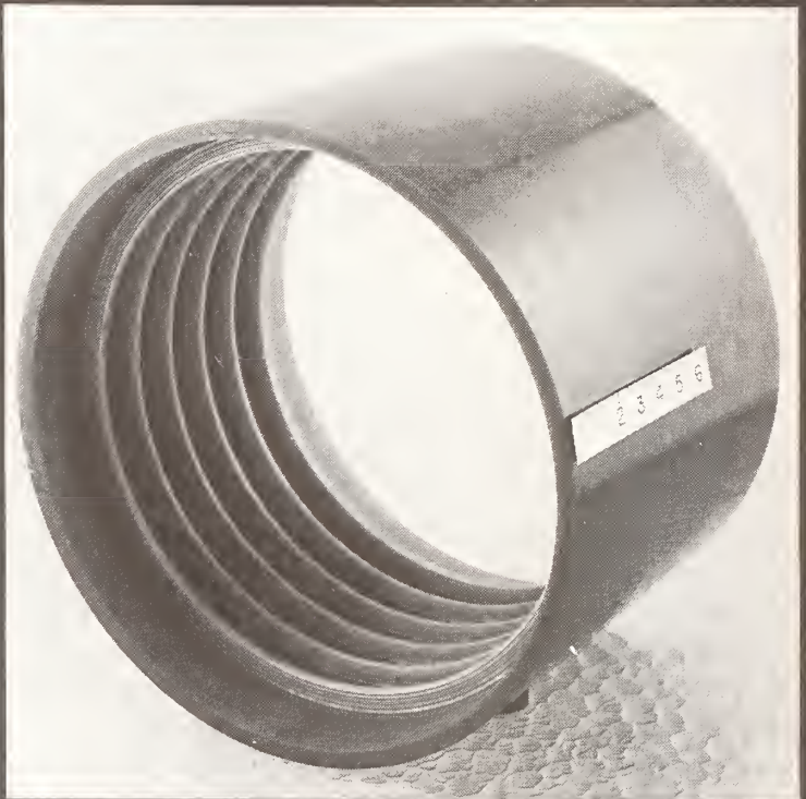
Figure 1. Composite Pressure Hull Prototype (1/22 - Scale)
