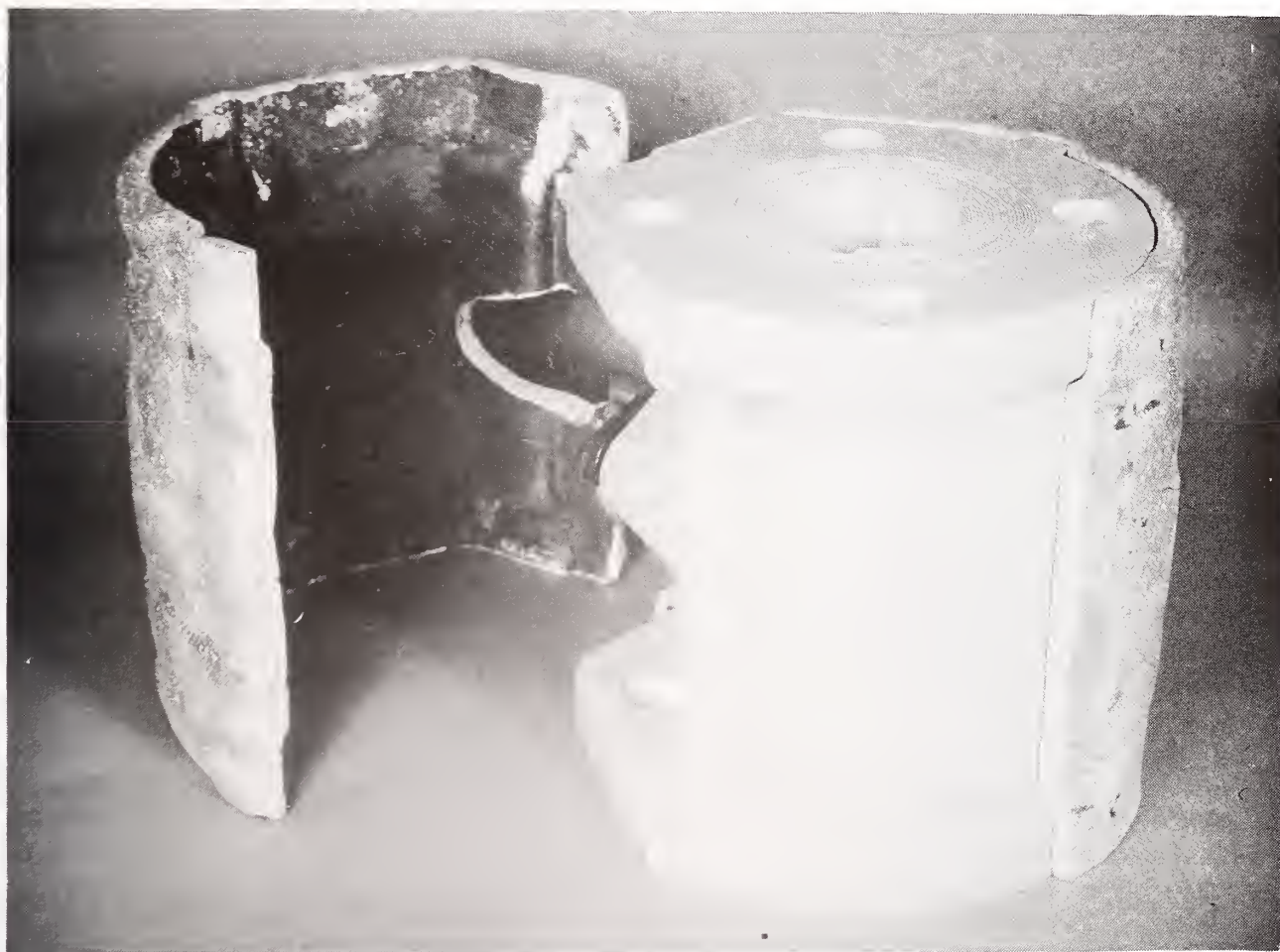
Figure 15. Composite Test Valve With Fire Shield
