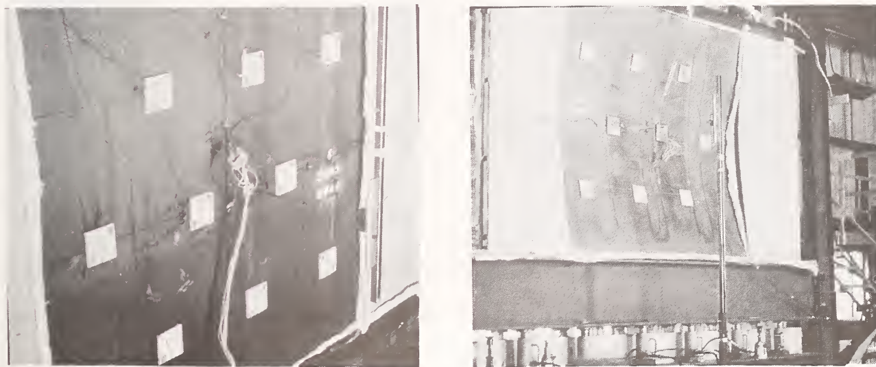
Figure 7. Two Composite Wall Sections in the ASTM E-119 Facility
