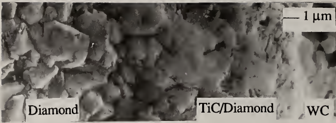
Fig. 2 SEM photograph of cross-section of multilayer diamond coating on WC with TiC as an interposing layer.
