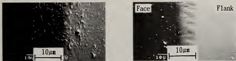
(a) 20% PCFRM (Cutting distance: 245m) (b) 20% MCFRM (Cutting distance: 245m)
