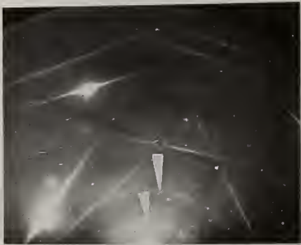
Fig. 3. Diamond particles on ends of irregular tips (a) and corresponding electron diffraction picture (b).
