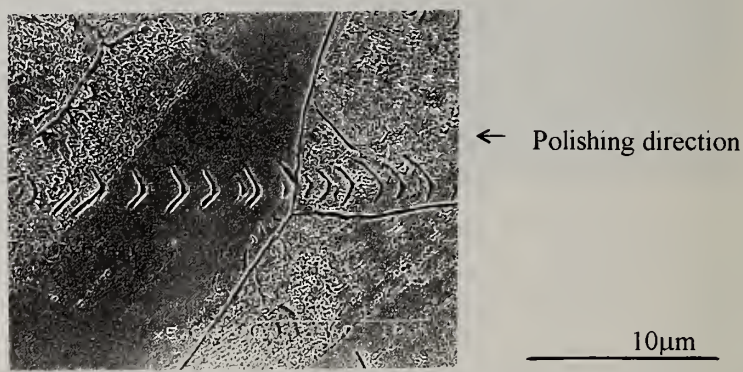
Fig.4 SEM photo of the etched CVD diamond surface polished with a #1500 wheel
