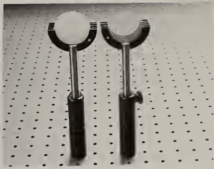
Fig. 1. Visibility through a large grain-size, translucent film on the left, is compared to visibility through a small grain-size, transparent film on the right.
