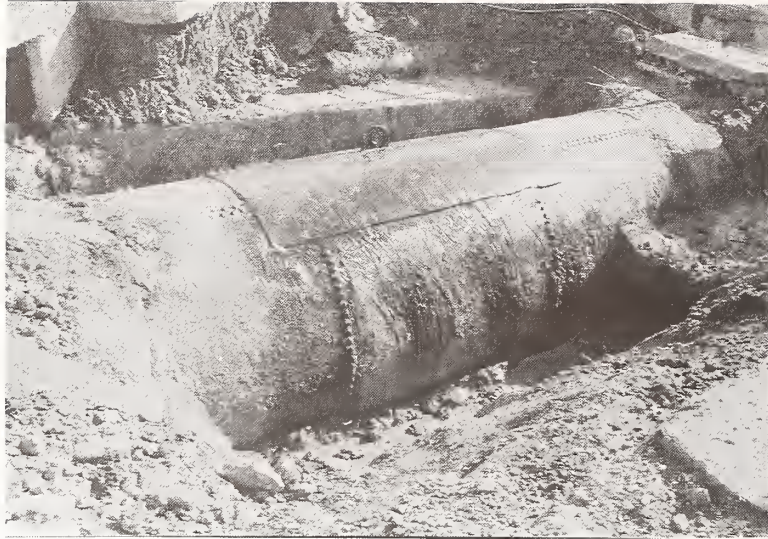
Photo 7.1 Rupture of a Main Water Pipe (Aqueducts Plant, DWP, City of Los Angeles)
