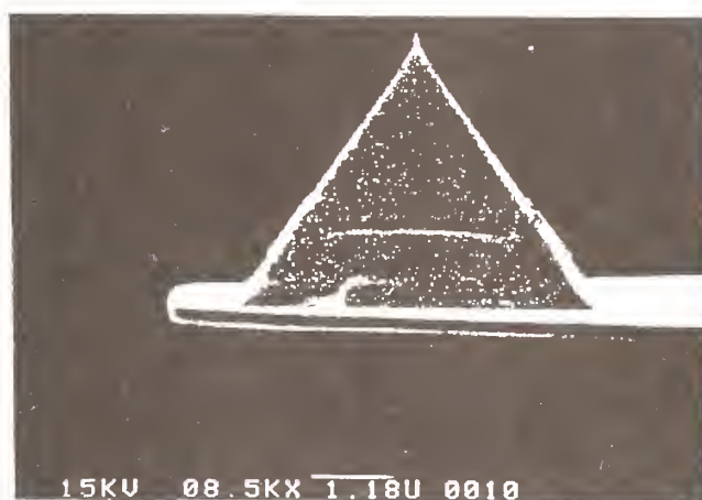
Fig.2 Sharpened pyramidal tip on the end of the cantilever
