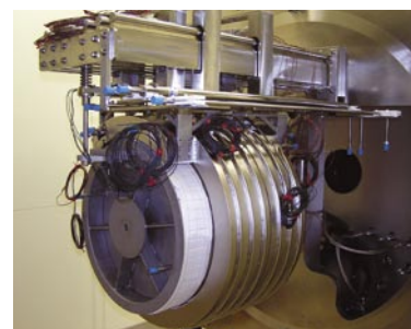
Front view of the Guarded Hot Plate (top), Installation of edge-guard assemblies, cold-plate assemblies, and hot plate (bottom).
