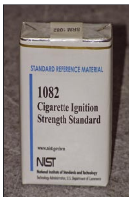
NIST's new SRM 1082 consists of 10 packs of cigarettes that have been specially made to be less likely to ignite household furnishings.
