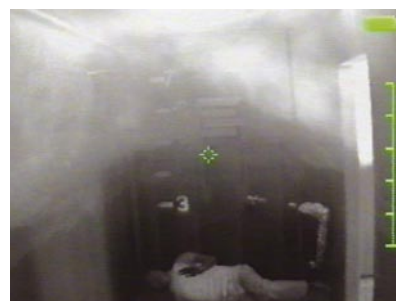
View of a corridor with a heated mannequin on the floor, and a temperature target and reflective strips on the back wall. Hot, smoke-laden gases are entering the corridor from an adjacent room on the right. The three TICs are viewing an identical scene at the same moment.
