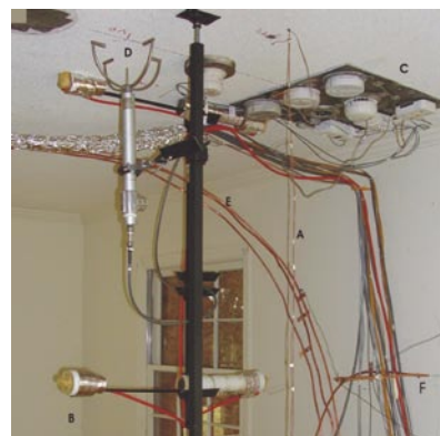
This photograph shows the wide range of instrumentation used to characterize the environment around smoke detectors during the recent investigation on home smoke alarms.
