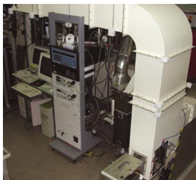
The Fire Emulator/Detector Evaluator.
