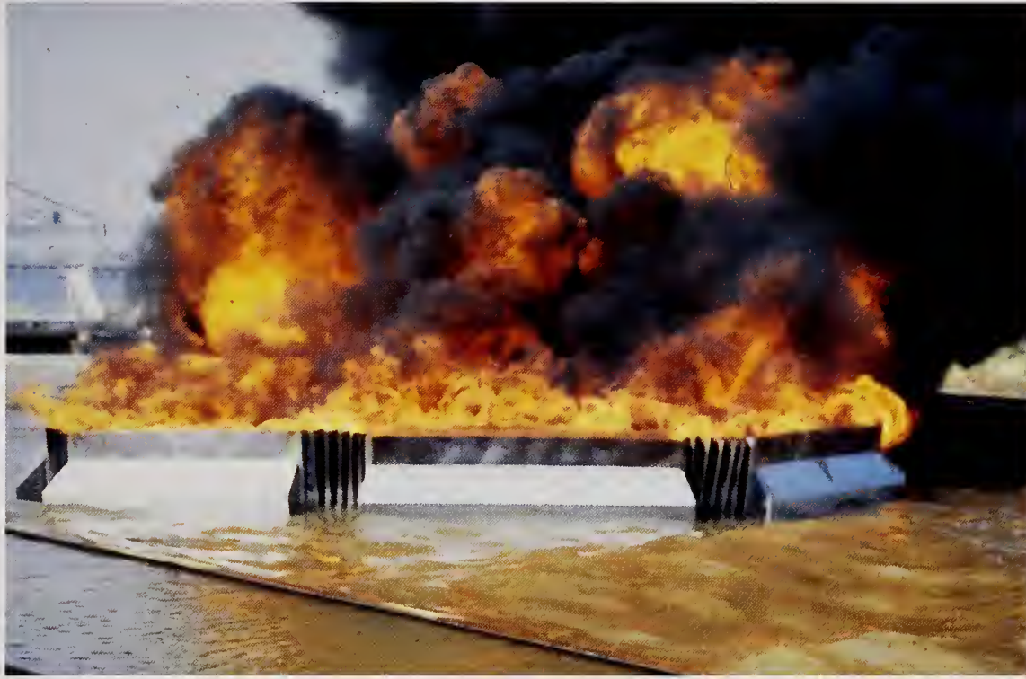
Fire test on oil spill containment boom
