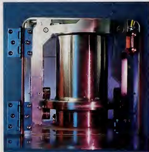
Gyrotory compactor for hot mix asphalt
