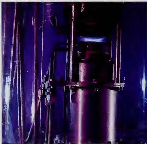
Stabilized flame for measuring refrigerant flammability
