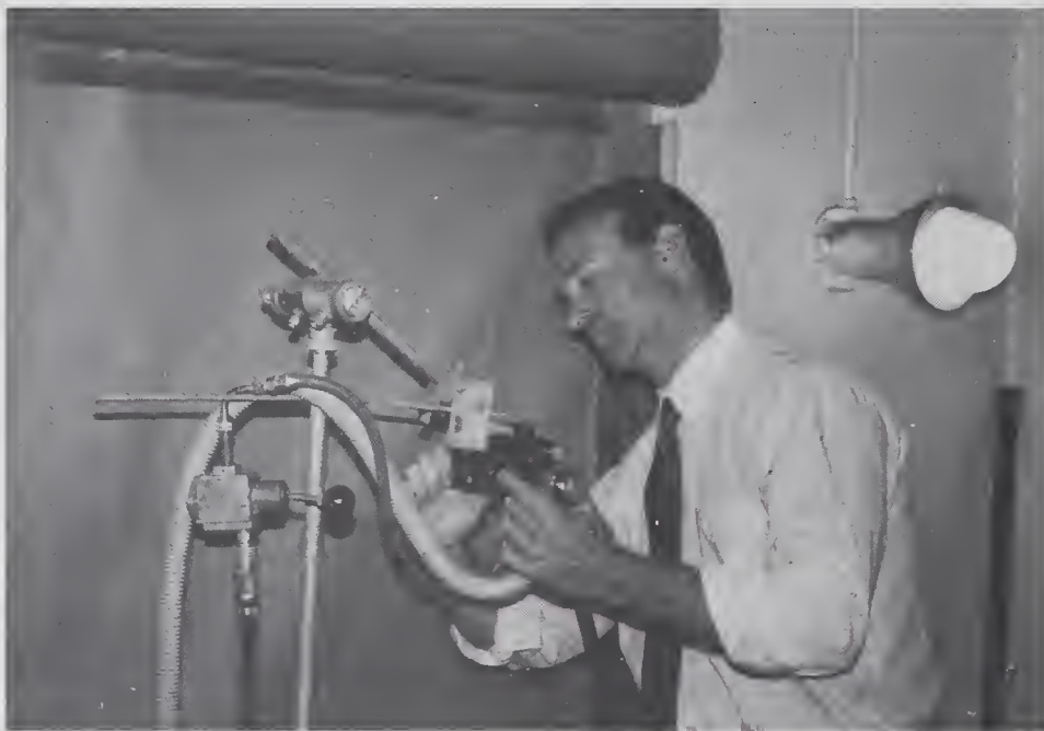
Figure 6. AccuSpray's Chief Engineer, Bob Amicarelli, preparing to shoot a test spray pattern with one of AccuSpray's new HVLP spray guns that are designed for continuous-duty spray applications.
