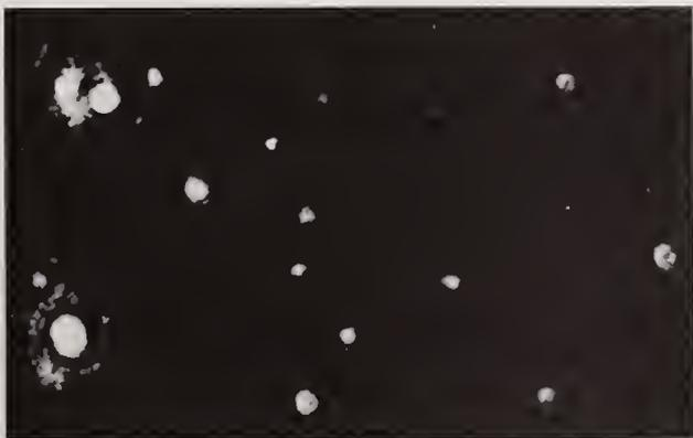
Fig.7 Reconstructed image of fuel droplet in Diesel spray.
