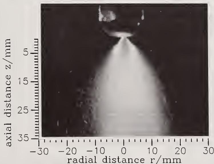
Fig. 3 Laser-light-sheet photograph
