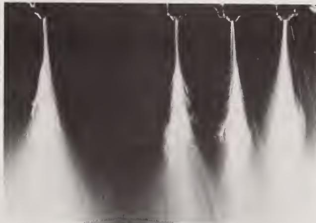
Fig 9. Comparison of edge profiles, LHS, single nozzle; RHS row configuration (6.8 aspect ratio)
