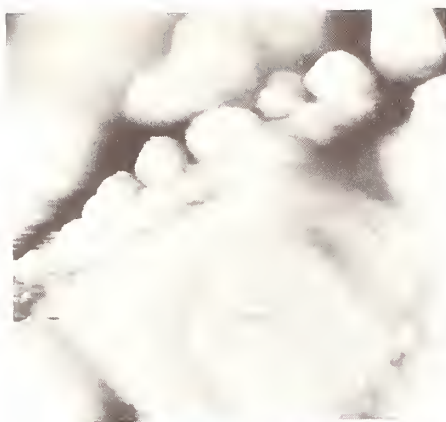
Fig. 1. Constant current image of the \text{ZnO}(000\bar{1}) face. Steps are visible which form (10\bar{1}0) and (11\bar{2}0) faces. The image is 771 \text{ \AA} \times 771 \text{ \AA} and was acquired at -1.5 \text{ V} sample bias and 0.3 \text{ nA} . The vertical resolution is 36 \text{ \AA} from black to white.
