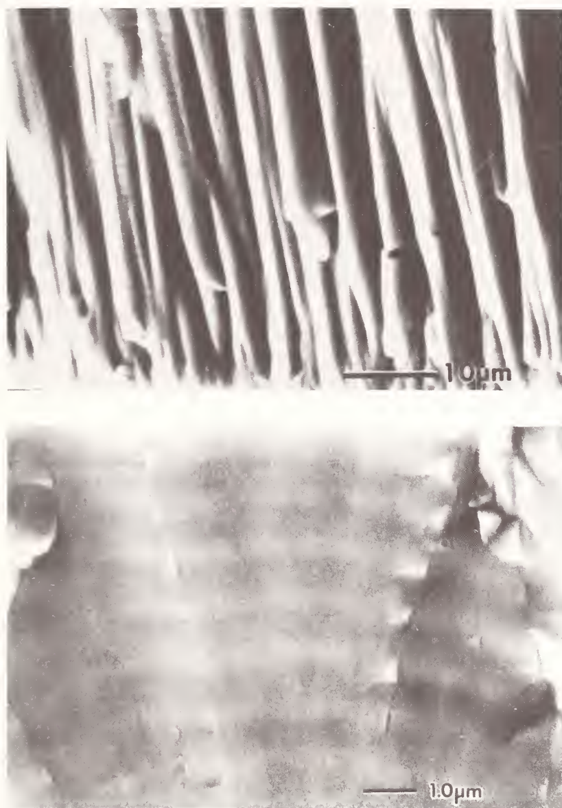
Figure 2. Scanning electron micrographs of modulated \text{Tl}_a\text{Pb}_b\text{O}_c/\text{Tl}_d\text{Pb}_e\text{O}_f films. Micrographs are low (top) and higher (bottom) magnifications of a cross-sectional view of a fractured film. Film was deposited by cycling electrode between 0.05 mA and 5 mA in a solution of 0.005 M \text{TlNO}_3 and 0.1 M \text{Pb}(\text{NO}_3)_2 in 5 M NaOH. Layer thicknesses are intentionally quite thick ( \sim 0.5 \mu\text{m} ) so that SEM imaging is possible.
