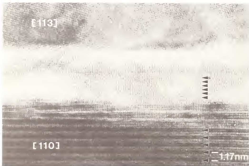
Figure 5. Micrograph of a grain boundary in \text{La}_{1.25}\text{Ba}_{1.75}\text{Cu}_3\text{O}_{7-\delta} , heated in nitrogen at 950^\circ\text{C} for 24 hours, showing the presence of \text{La}_{2-x}\text{Ba}_x\text{CuO}_4 at the grain boundary. When this material is heated in oxygen atmosphere no second phase is formed.
