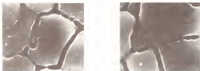
Figure 3 SEM photographs of the etched surfaces. The surface was chemically etched by 20wt% phosphoric acid after thermal etching.
