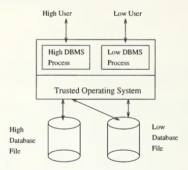
Figure 6: TCB Subset Architecture.
