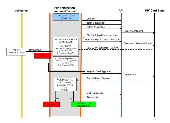
Figure B-6. Authentication using an asymmetric Card Authentication Key
