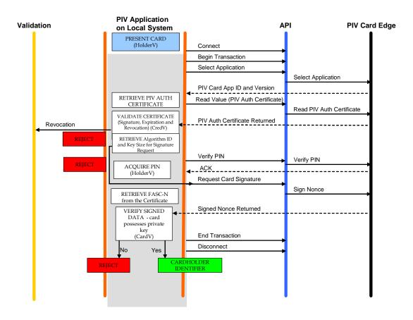
Figure B-5. Authentication using PIV Authentication Key
