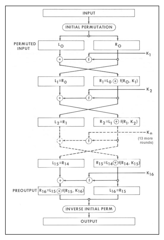
Figure 1. Forward Transformation of the DEA Cryptographic Engine
