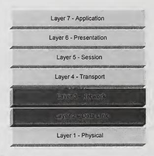
Figure 2.3: OSI Layers Addressed by Packet Filters
