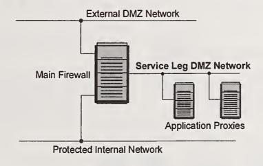
Figure 3.2: Service Leg DMZ Configuration
