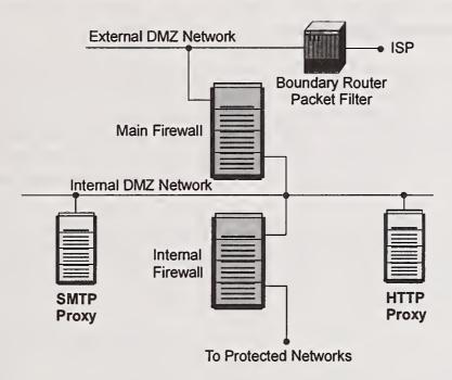
Figure 2.8: Application Proxy Configuration
