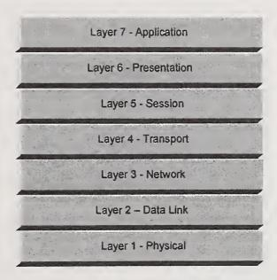
Figure 2.1: OSI Communications Stack
