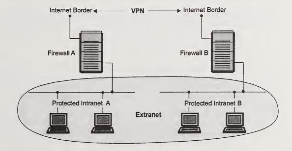
Figure 3.4: VPN/Extranet Joining Two Intranets
