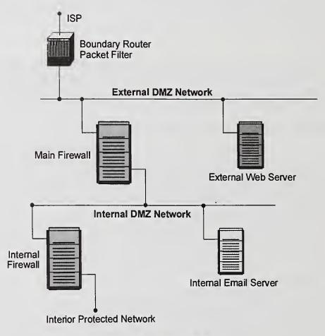
Figure 3.1: A DMZ Firewall Environment
