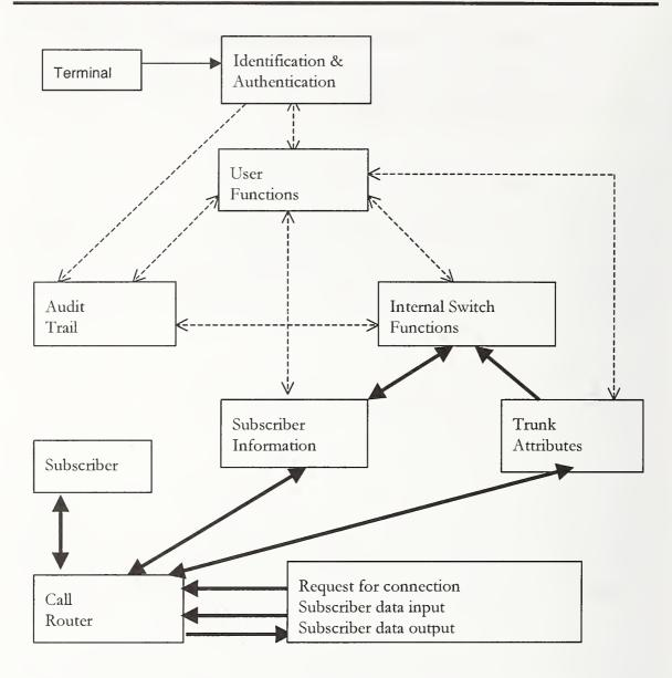
Figure 2. PBX Functional Architecture
