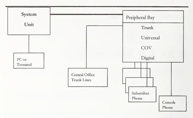
Figure 1. PBX Block Diagram
