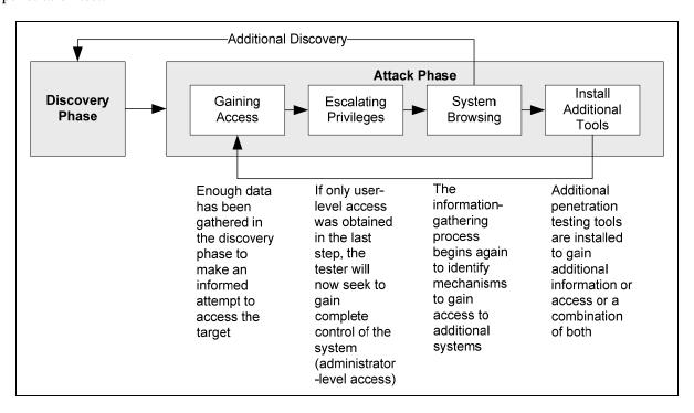
Figure 5-2. Attack Phase Steps with Loopback to Discovery Phase
