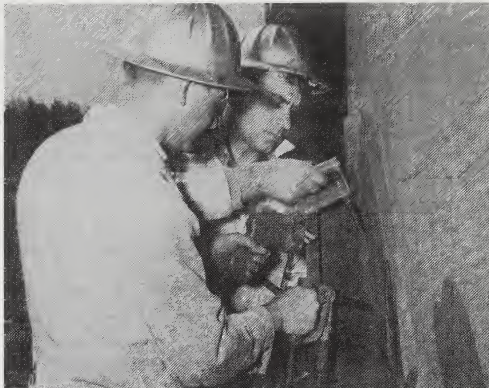
Examining a welded tank by magnetic particle method (From: Principles of Magnetic Particle Testing, MAGNAFLUX, 1985)
