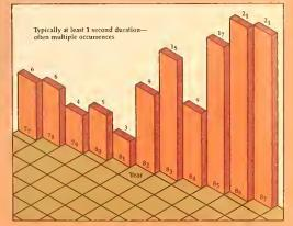
This chart shows only those outages lasting long enough to disturb electromechanical equipment. Electronic equipment can be disturbed by much shorter (and more frequent) outages.
