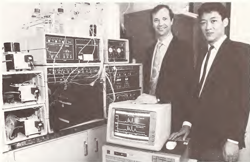
A collaborative effort between NIST and Dionex Corp. resulted in the development of a new generation of a widely used analytical chemistry instrument. H.M. (Skip) Kingston of NIST (left) and Archava Siriraks of Dionex are shown with the chelation ion chromatography system.
