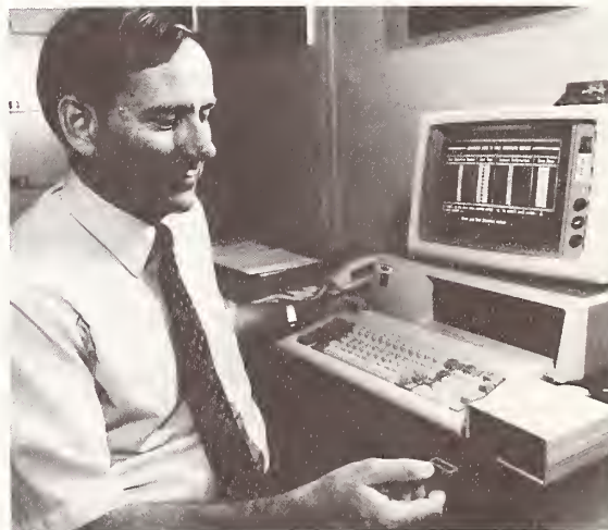
Before logging onto a network, Miles Smid uses a credit card-sized board, called a "smart" token, to perform a series of authentication checks for security.
