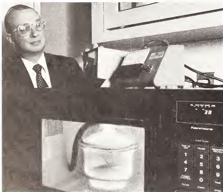
John A. Tesk sterilizes clinical instruments with a new microwave-generated gas plasma method. The new technique may reduce the damage to expensive instruments caused by repeated exposure to time-consuming, traditional sterilization methods.
