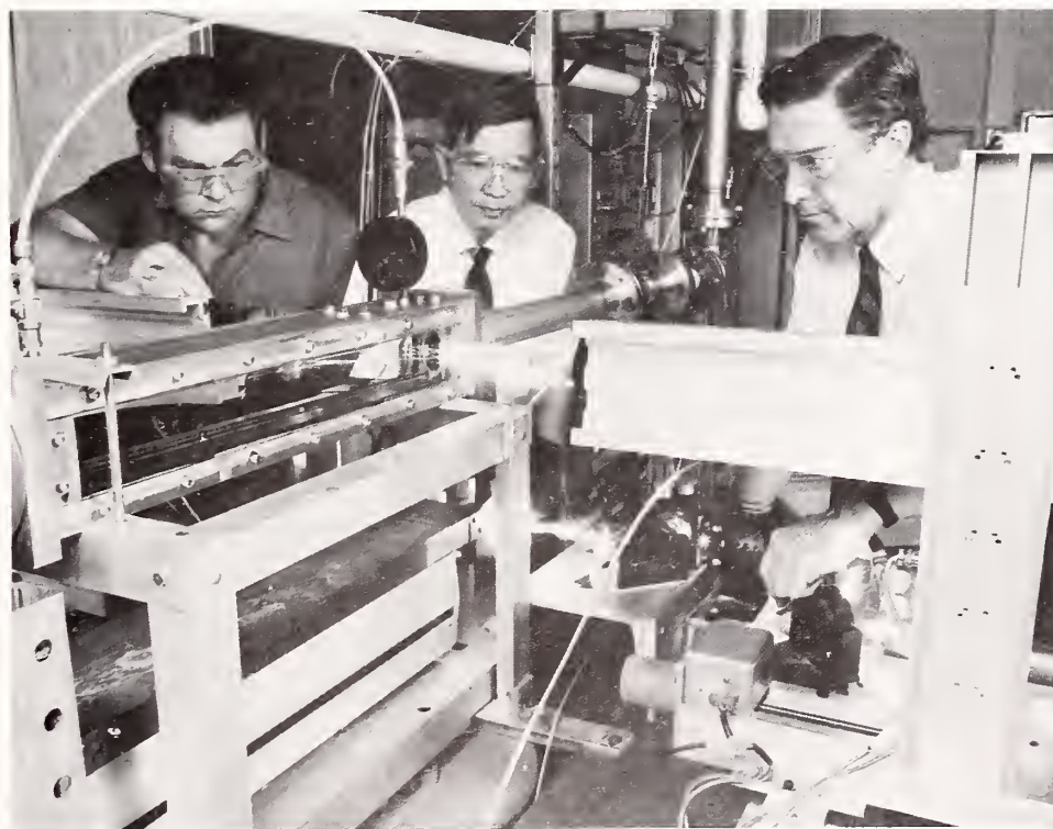
Mechanical engineers George Mattingly (right) and T.T. Yeh (center), with technician Boyd Shomaker, study flow-measuring devices using laser Doppler velocimetry at the NIST fluid metering research facility.
