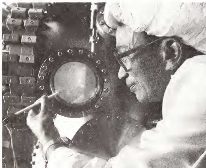
Wen Tseng, materials research engineer, observes an in-situ reflection electron diffraction pattern during the growth of gallium arsenide.
