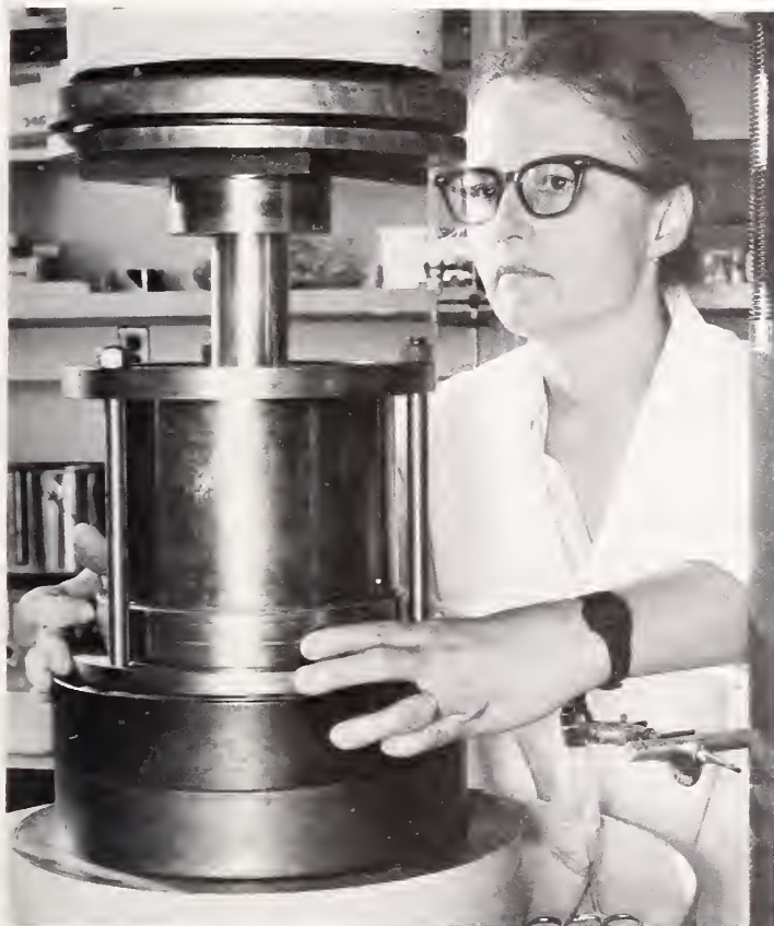
Materials research engineer Leslie Struble uses a cylinder and piston device to study the causes of concrete failure.
