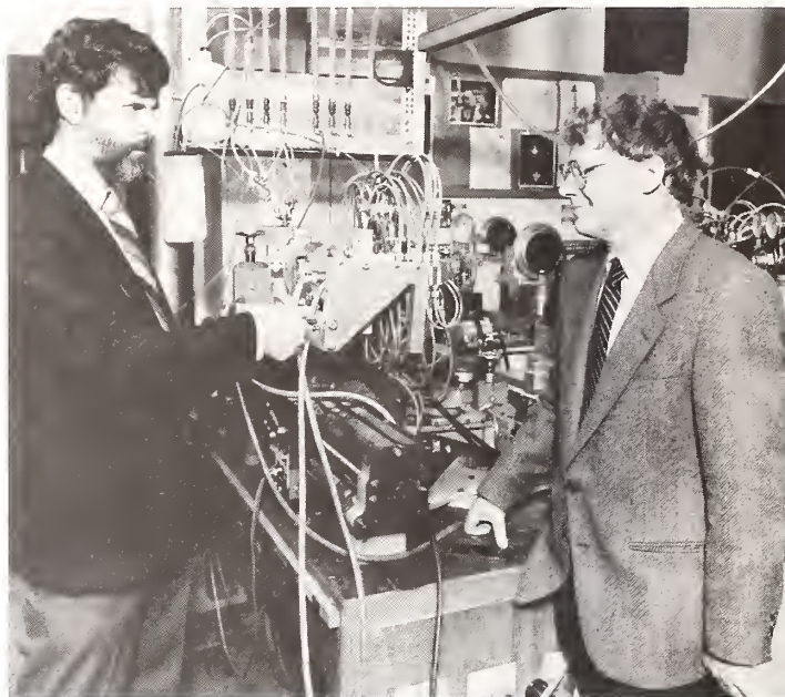
Jeffrey Fuhr (left), a physicist in the NIST Atomic Transition Probabilities Data Center, demonstrates the wall-stabilized arc to W.L. Wiese, head of the data center. The arc is used to measure atomic transition probabilities for use in plasma modeling and analysis, including fusion research as well as laser physics and astrophysics.
