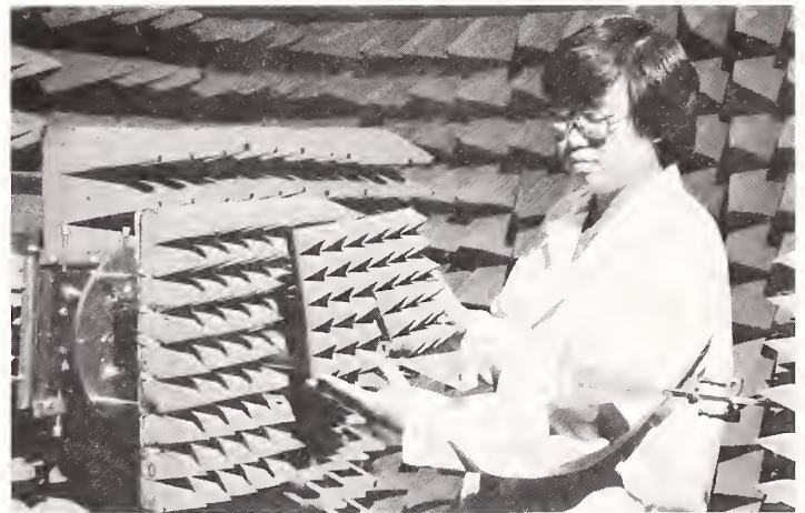
Douglas T. Tamura, an electronics technician, aligns antennas being calibrated on the extrapolation range, which is part of the near-field antenna measurement facility.
