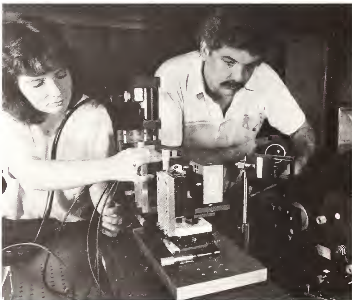
On the automated spectral comparator facility, physicists Jeanne Houston and Chris Cromer align the silicon photodiode light traps that are used in photodetector research and calibration.
