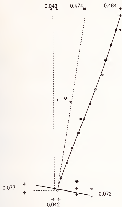
Figure 5 Measured and computed mode shape for the first E-W mode after retrofit
