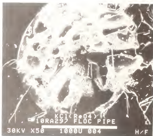
Figure 4. Scanning electron micrograph of defect in a \text{KCl}(\text{ReO}_4) crystal grown from melt with 2.5 mol % \text{KReO}_4 .
