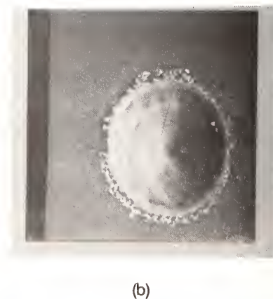
Figure 5. Electron micrographs of catastrophic damage in ZnSe; (a), crater showing coalescence of pits around the edges; (b), single pit showing fracture lines at the bottom.
