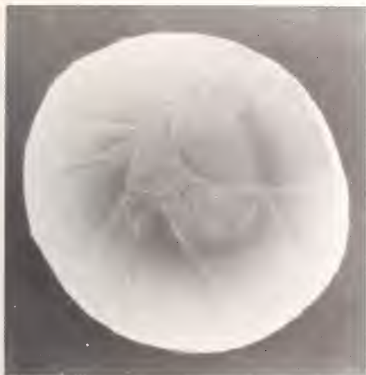
Figure 5. High inclusion density zones and grain boundaries in heavily doped \text{KCl}(\text{ReO}_4) crystal.
