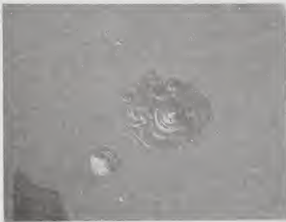
Figure 2. Typical Damage Site Above Threshold. 250X Nomarski micrograph of Sample 2 showing evolution from small damage pits through larger damage pits to crater. Large crater is approximately 100\ \mu\text{m} in diameter. Note the high quality surface finish.
