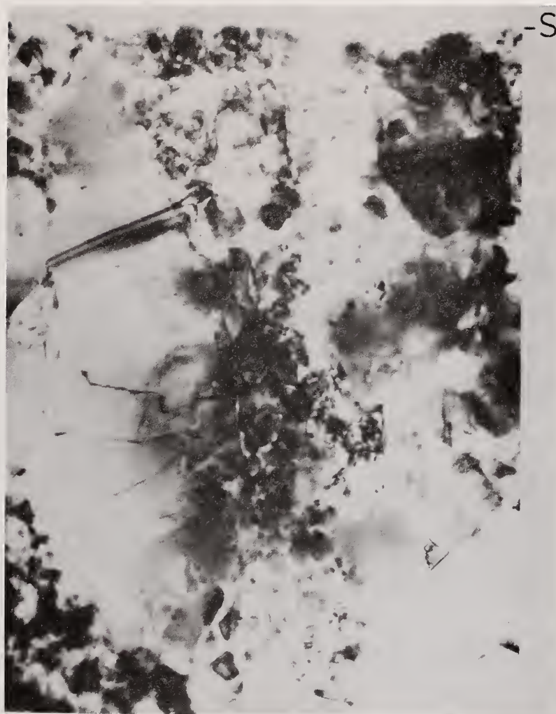
Figure 7 Cross sectional transmission electron micrograph of lead fluoride film deposited at ambient temperatures showing its composite character, with residual porosity in intergranular regions.
