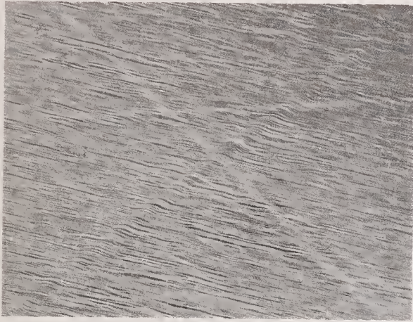
Figure 4. Sample 11 Surface, "Good" Region. 250X Nomarski micrograph showing residual polishing marks. Note fine structure approximately parallel to c axis.
