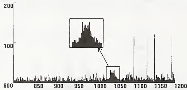
**Fig. 3. Frame-to-frame Difference based on Histogram Intersection.**
