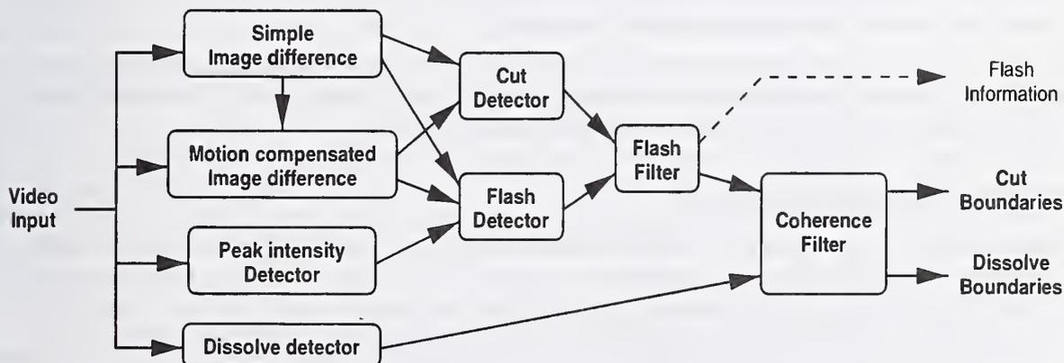
Figure 1: System architecture
