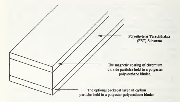
Figure 1. 3480 Type Tape Structure.
