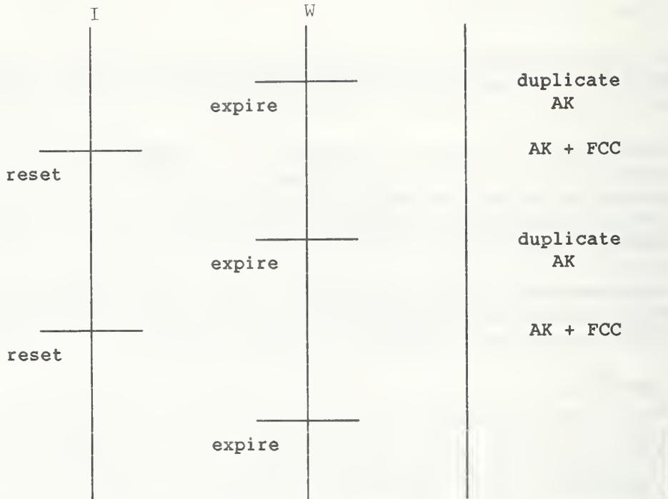
Figure 1 - ACK exchange on idle connection.
