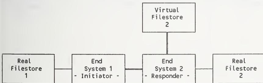
**Figure 1 - Model of file transfer/access.**
