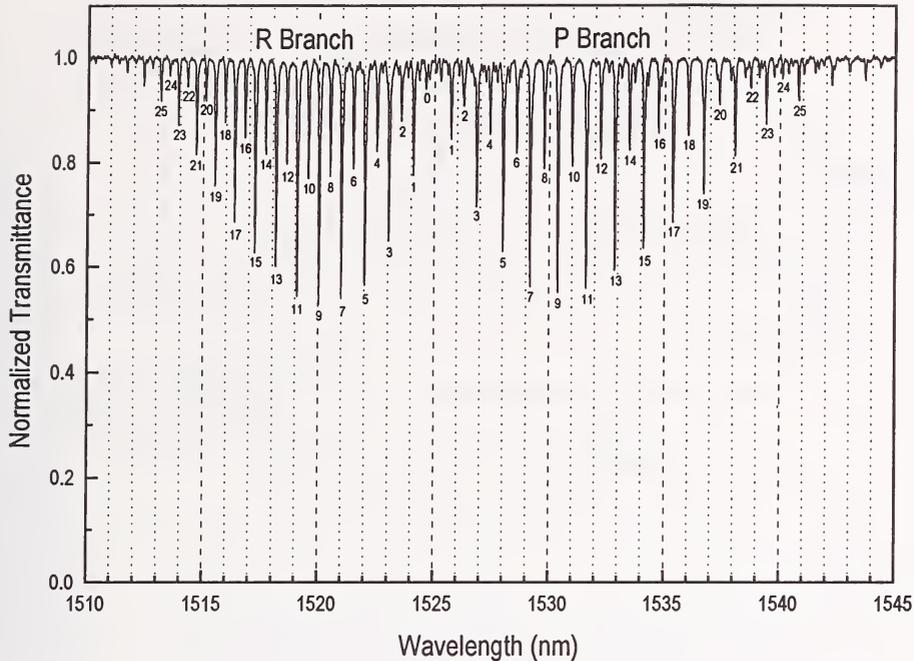
**Figure 1.** Acetylene ( $^{12}\text{C}_2\text{H}_2$ ) spectrum taken by passing LED light through an absorption cell and recording the spectrum of the transmitted light using an optical spectrum analyzer with 0.05 nm resolution. This spectrum has been divided by the LED spectrum.
