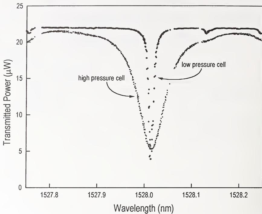
Figure 4. Scan over line P5 showing transmission through low pressure and high pressure cells.
