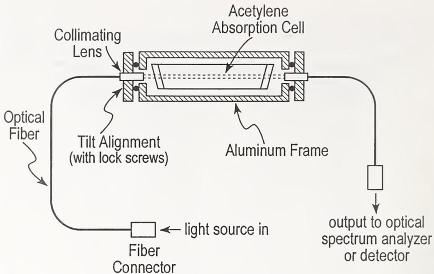
Figure 2. Schematic of fiber-pigtailed cell holder.
