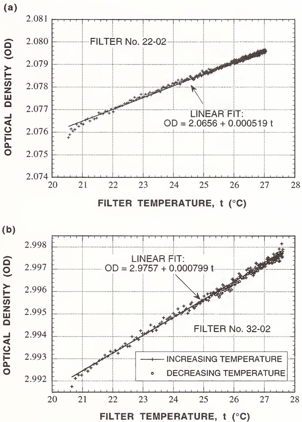
Figure 5. Optical density versus filter temperature for two filters:
