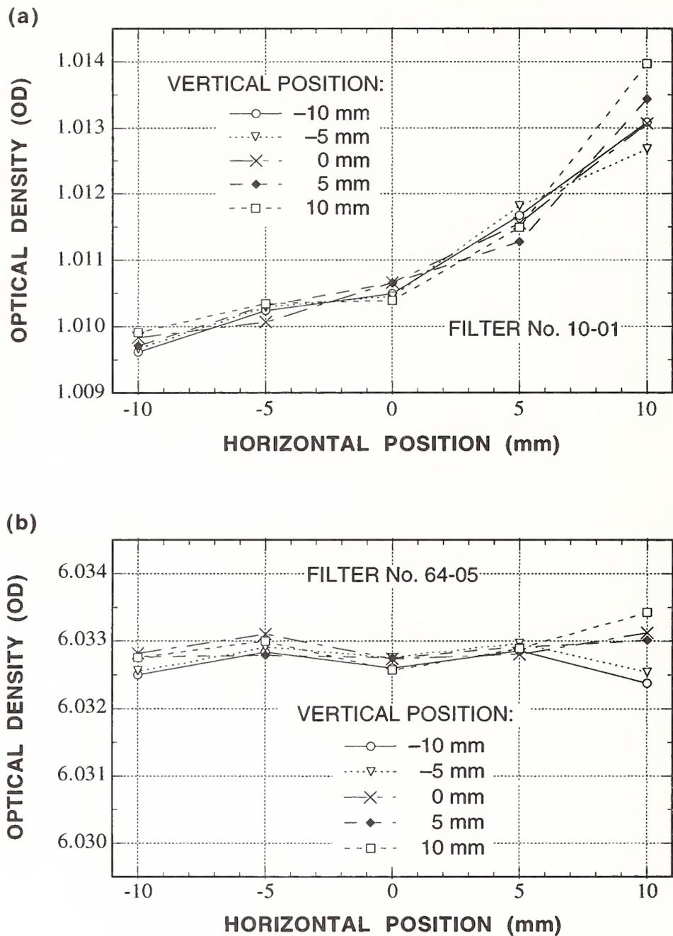
Figure 6. Spatial variation of the optical density for two filters, where the positions are measured from the center of the filter: a) Nominal OD = 1, relatively poor spatial uniformity; b) Nominal OD = 6, relatively good spatial uniformity.
