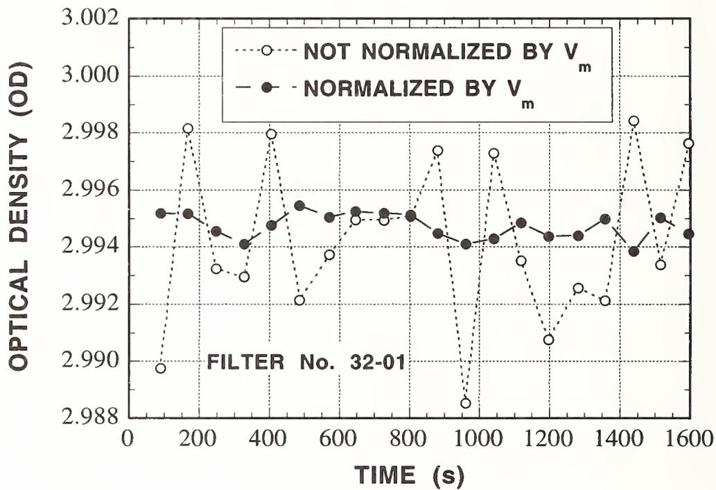
Figure 4. Comparison of the optical density calculated with and without normalization using the monitor detector output.
