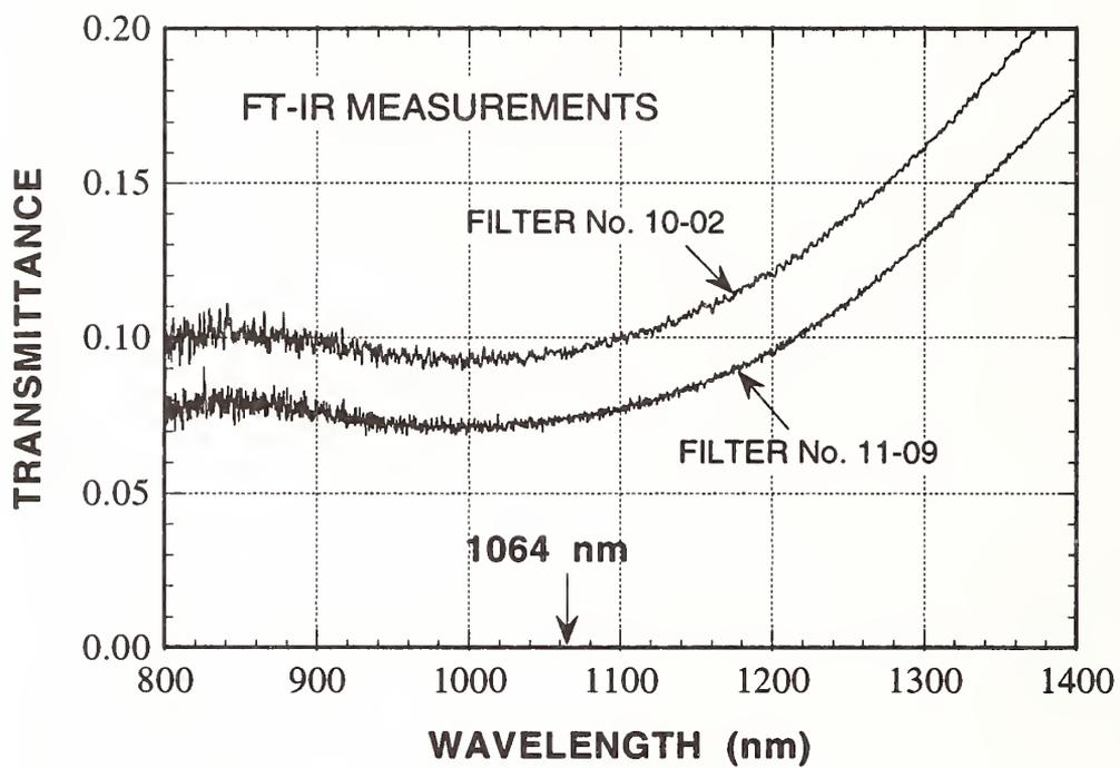
Figure 8. Transmittance in the region from 800 nm to 1400 nm of two filters measured using a Fourier transform infrared spectrometer.
