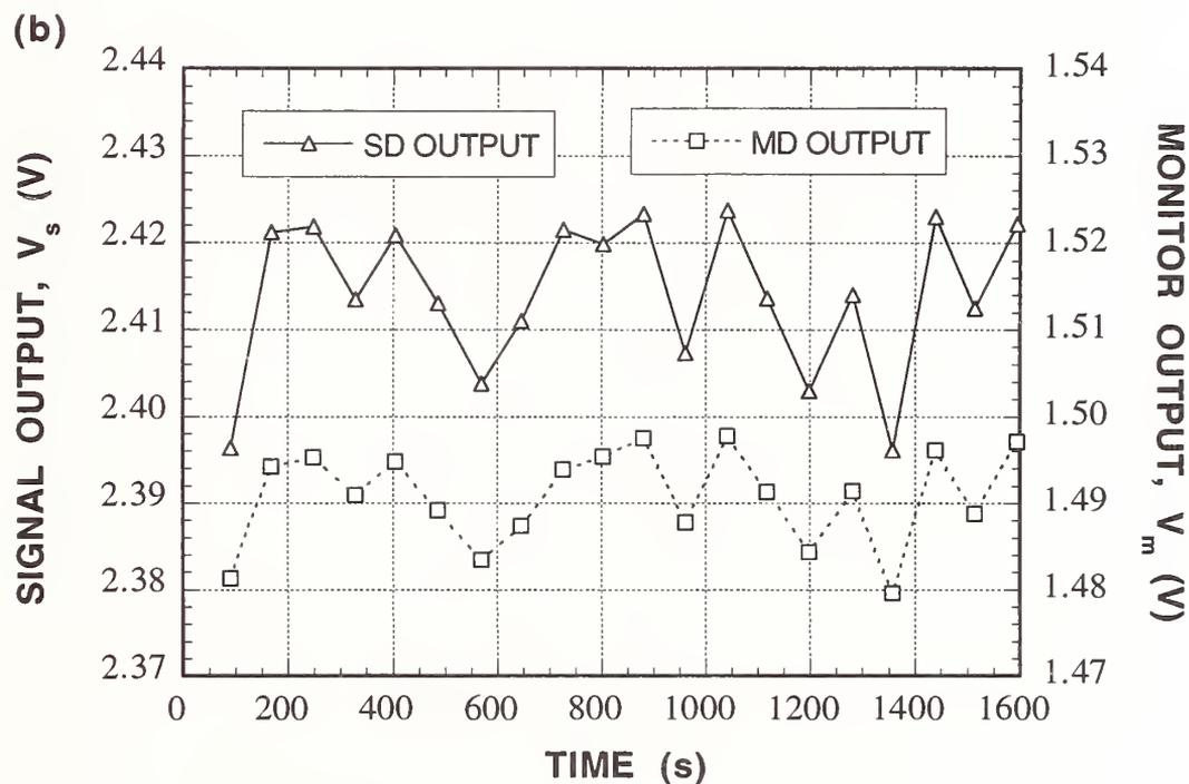
Figure 3. Outputs from the signal detector and the monitor detector during measurements when the laser beam passes through the reference. The laser power is more stable in a) than in b).
