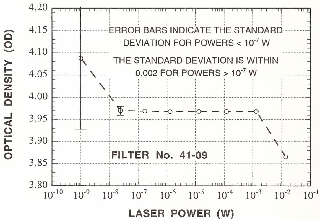
Figure 2. Optical density of a filter (nominal OD = 4) measured with different laser powers.
