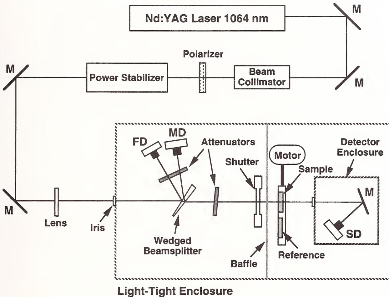
Figure 1. Schematic of the optical setup for transmittance measurements at 1064 nm wavelength, where M represents mirror; FD = feedback detector; MD = monitor detector; SD = signal detector.
